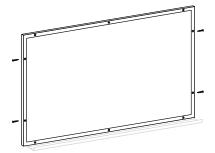
Install the self-tapping screws (supplied with the board) through the pre-drilled holes in the trim. Clean the board thoroughly before using. See markerboard care and maintenance instructions.
