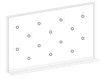
Prepare the surface of the existing board by thoroughly cleaning it of dirt, dust, or grease. Apply construction adhesive to the surface of the existing board in golf-ball size amounts every 16" in height and every 24" in length.
