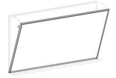
Position the new board carefully over existing board, and press firmly in the locations of the adhesive.
